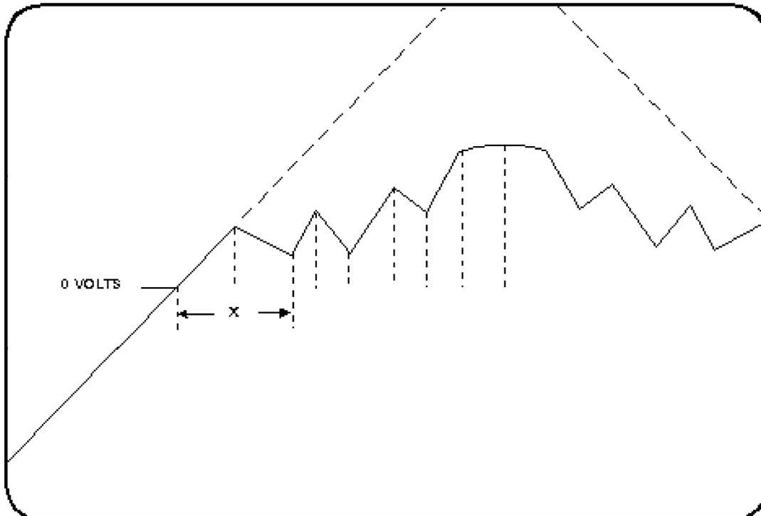
Figure 4-6: Output of Linearizer on Oscilloscope Screen Using Triangle Wave
