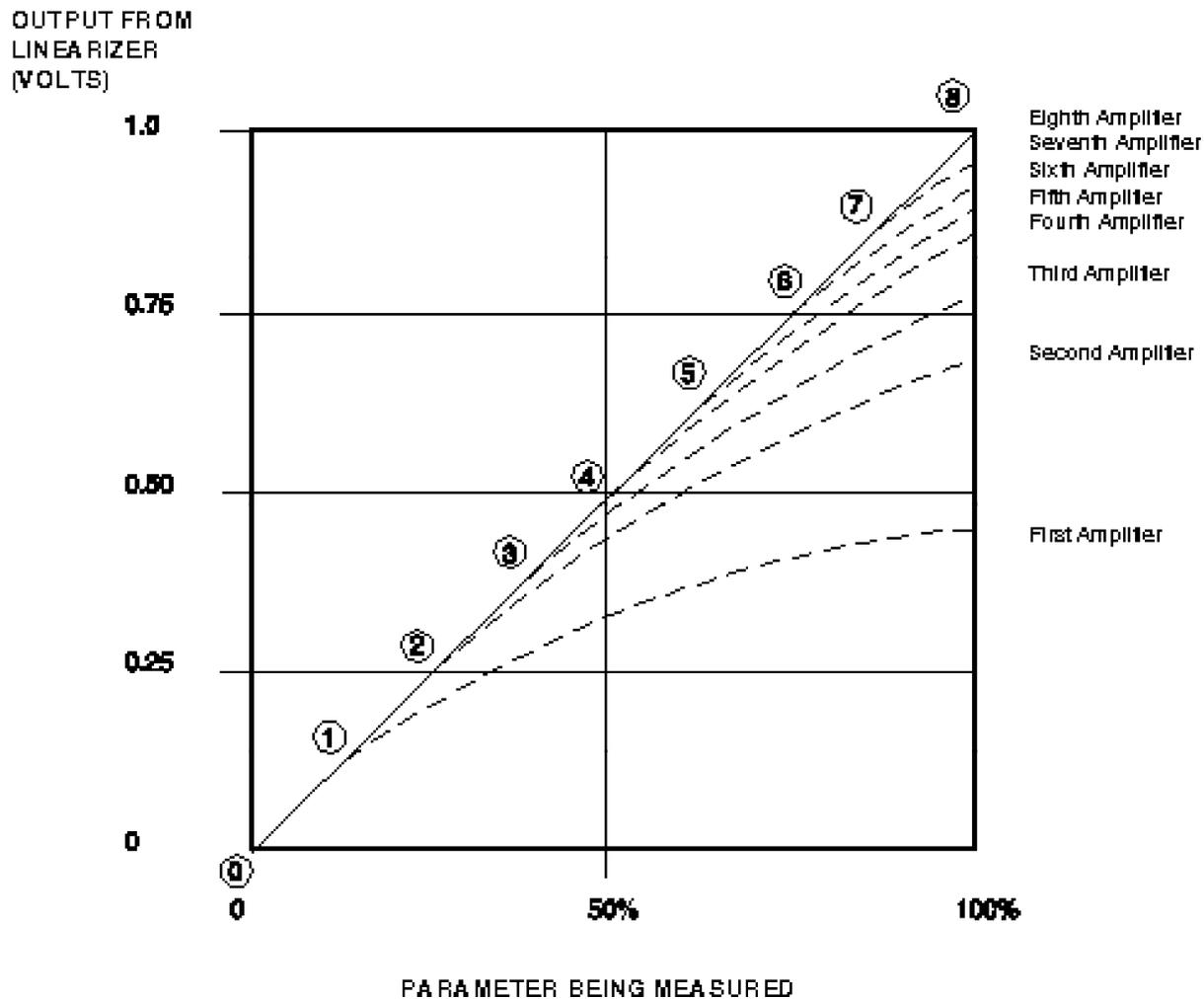
Figure 4-4: The Effect of Each Amplifier on the Final Result
