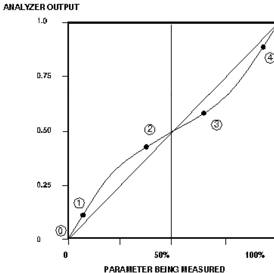
Figure 4-9: An "S" Shaped Curve
