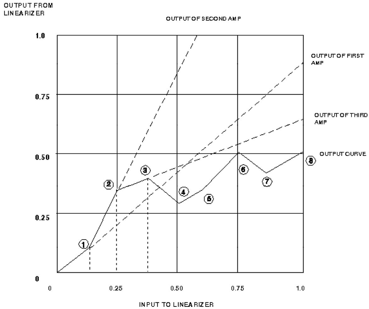
Figure 4-5: Exaggerated Illustration of How the Linearizer Works
