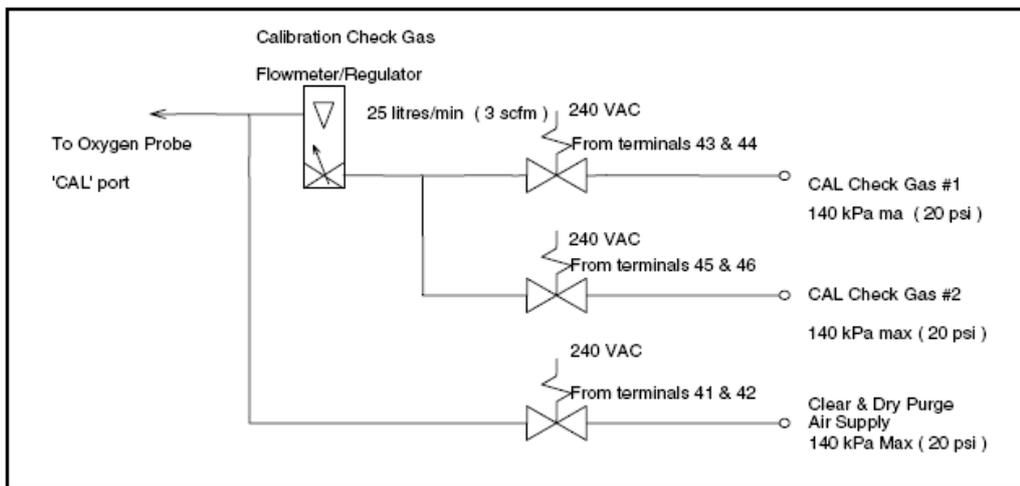
Automatic Purge & Calibration Check System Piping Schematic
