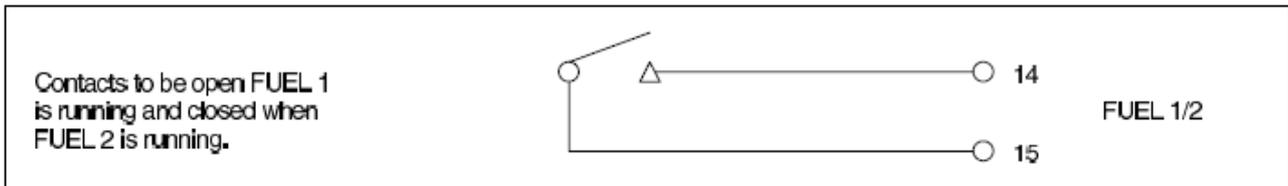
Fuel Selector Input Contact Connection
