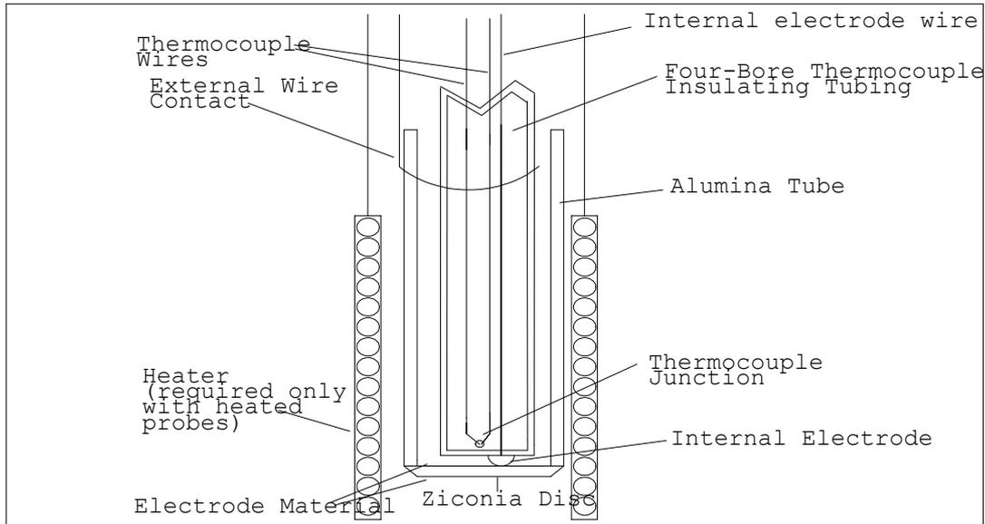
**Fig 2.1 Schematic View of a Sensor Assembly**
