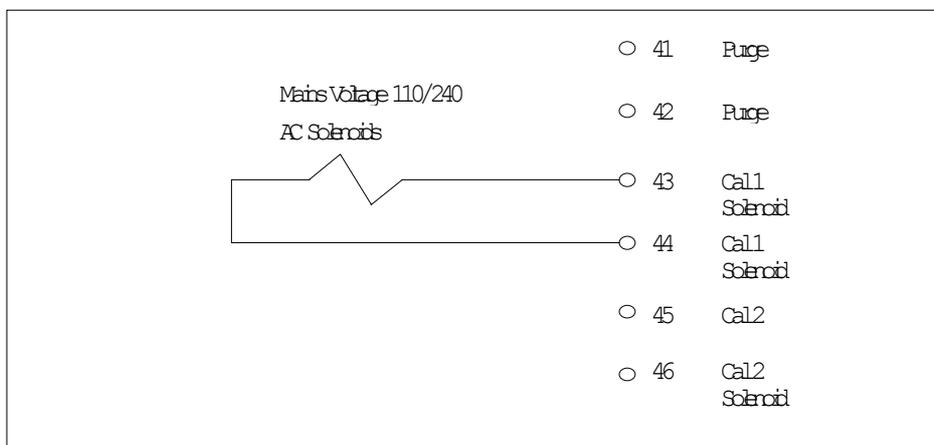
Figure 3.5 Automatic Oxygen Calibration check Solenoid Connection
