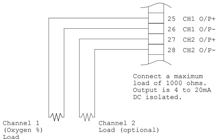
**Figure 3.4 Connections for Transmitter Output Channels.**
