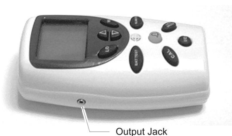
Figure 2-9: 0-1 VDC or RS 232 Digital Output Port
