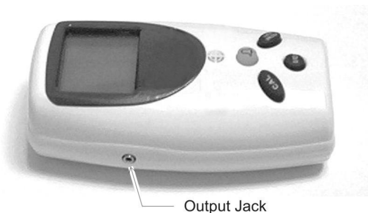
Figure 2-8: 0-1 VDC or RS 232 Digital Output Port
