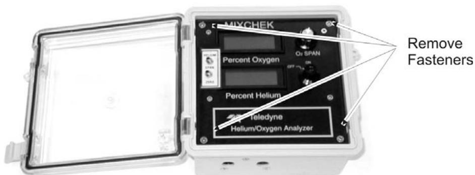
*Figure 2-2: Removing the Front Panel
