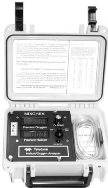
Figure 1-2: MIXCHEK—Portable Configuration
