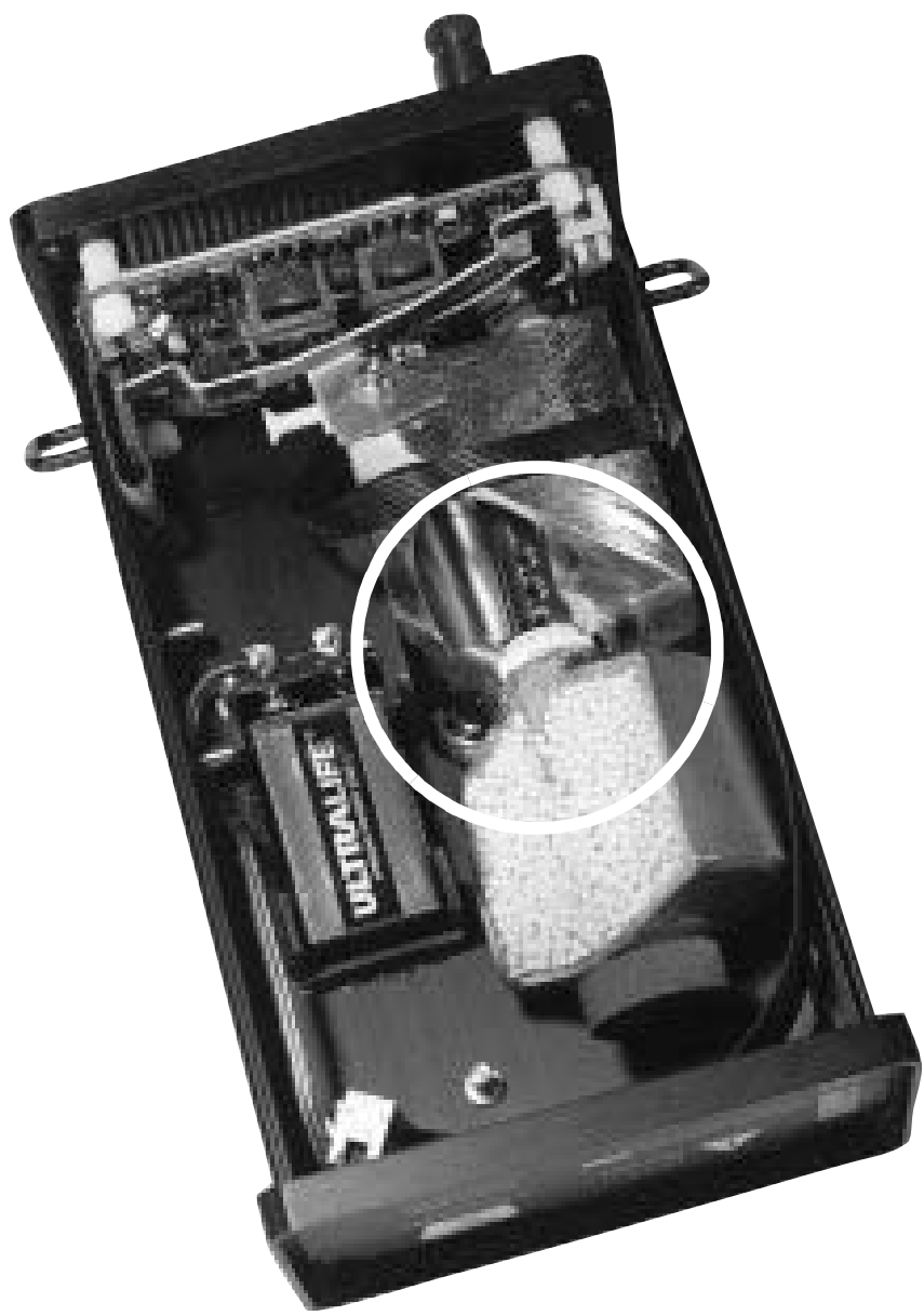
Bottom view of 8800P with cover open. The sample chamber and desiccant cartridge are shown cut open to facilitate an understanding of the mechanism and how it is assembled.
