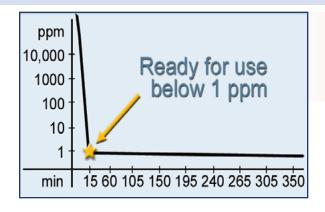
Using Teledyne's Insta Trace technology, meaningful readings below 1 ppm are obtained in only 15 minutes.
