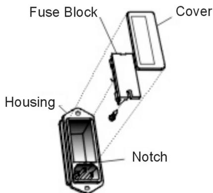
To change between American and European fuses, remove the single retaining screw, flip fuse block over 180 degrees, and replace screw.
