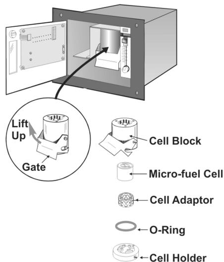
**CAUTION:** THE CELL IS SHIPPED SEPARATELY INSIDE TWO BAGS FILLED WITH OXYGEN-FREE INERT GAS. USE CARE TO AVOID EXPOSING THE CELL TO AIR FOR ANY LONGER THEN NECESSARY TO INSTALL THE ITEM.
