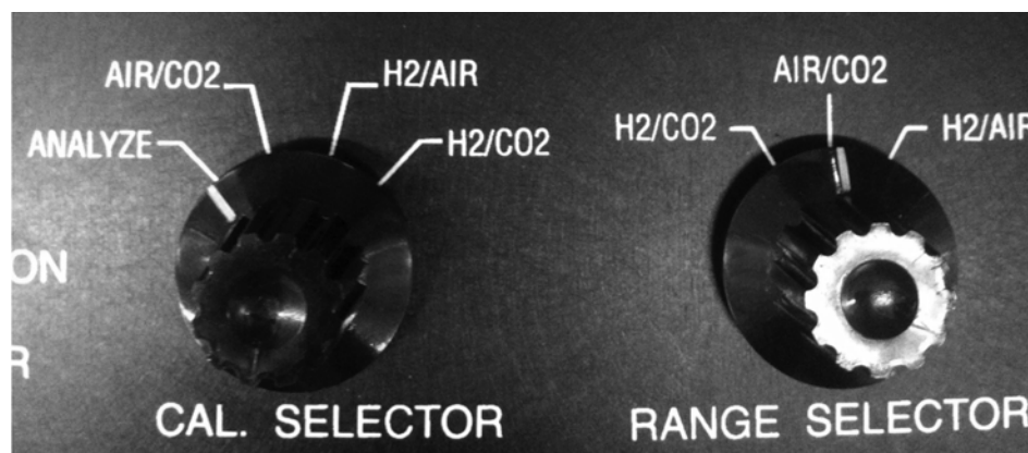
Figure 3-8: Range Switch in AIR/CO2 Position
