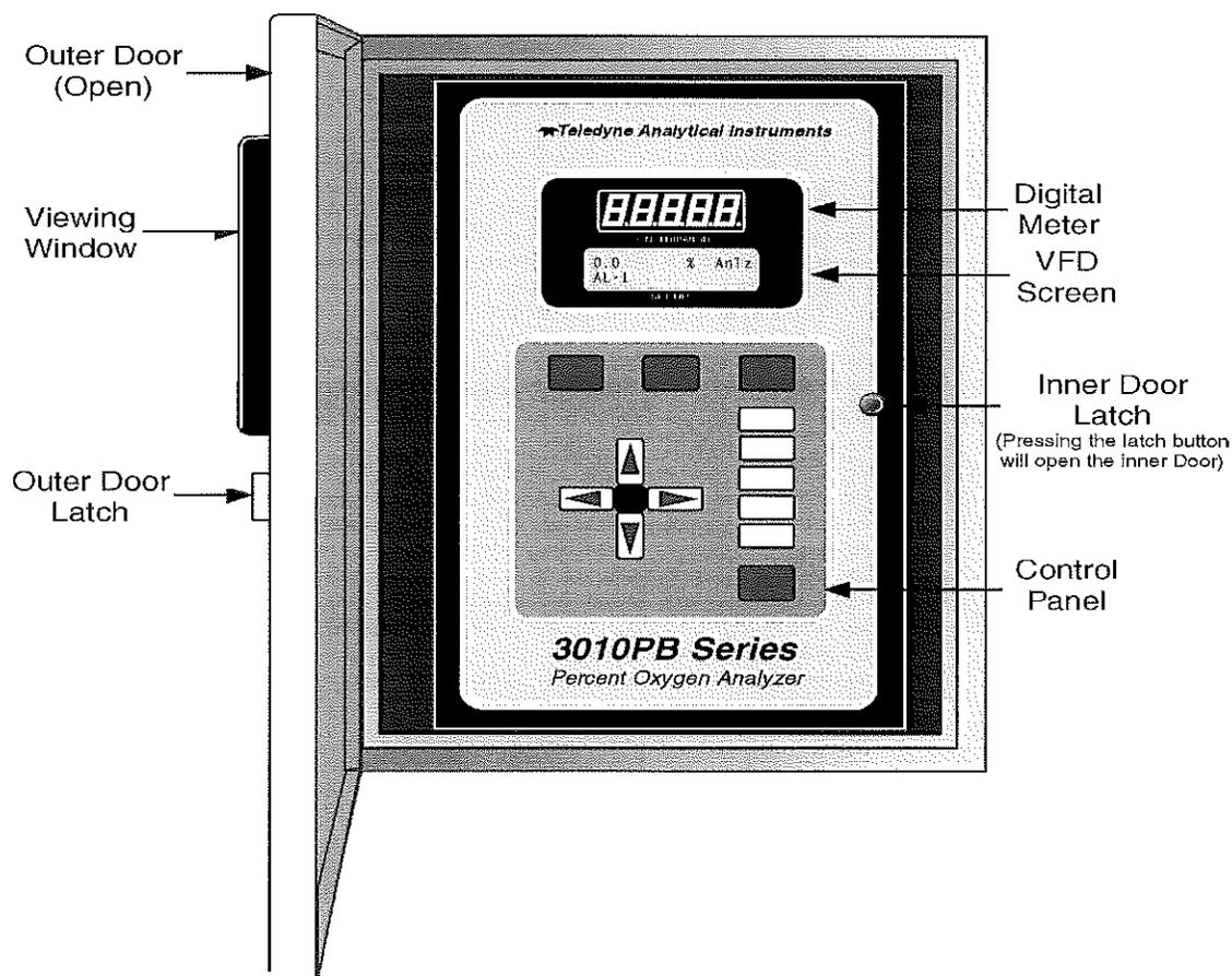
Figure 1-1: Front of Unmounted Control Unit
