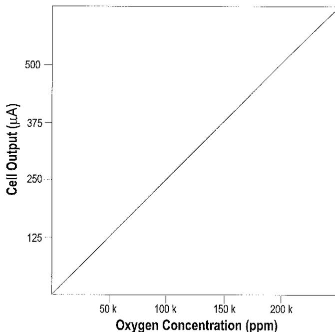
Figure 2-3. Characteristic Input/Output Curve for a Micro-Fuel Cell
