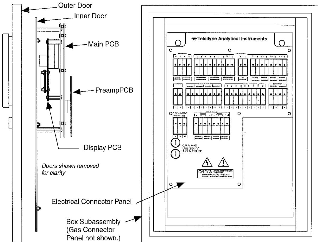
Figure 5-3: Control Unit Major Internal Components
