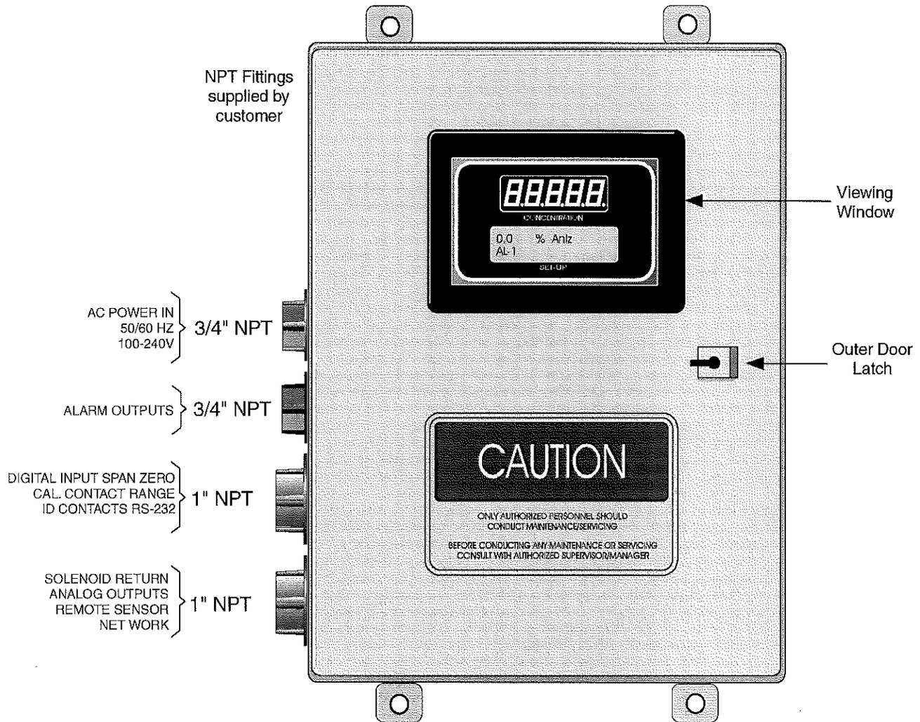
All operator controls are mounted on the inner control panel, which is hinged on the left edge and doubles as a door to provide access to the internal components of the instrument. The door will swing open when the
