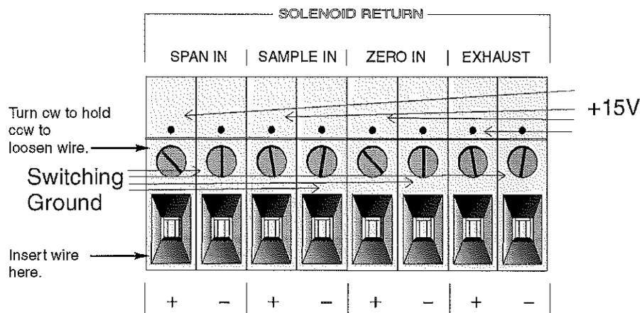
Figure 3-8: Remote Probe Connector Pinouts
