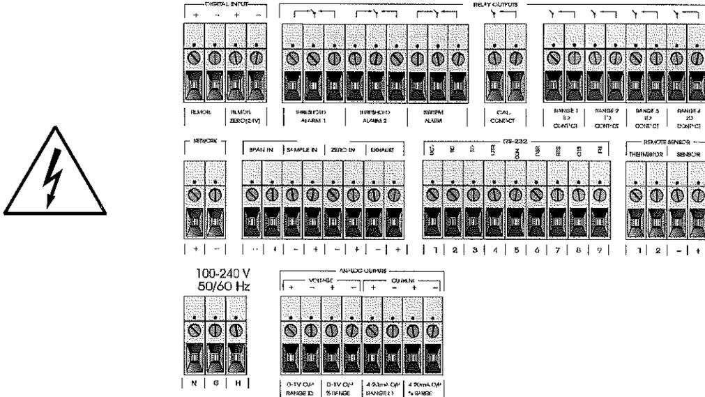
Figure 3-3: Interface Panel of the Model 3010PBC Control Unit
