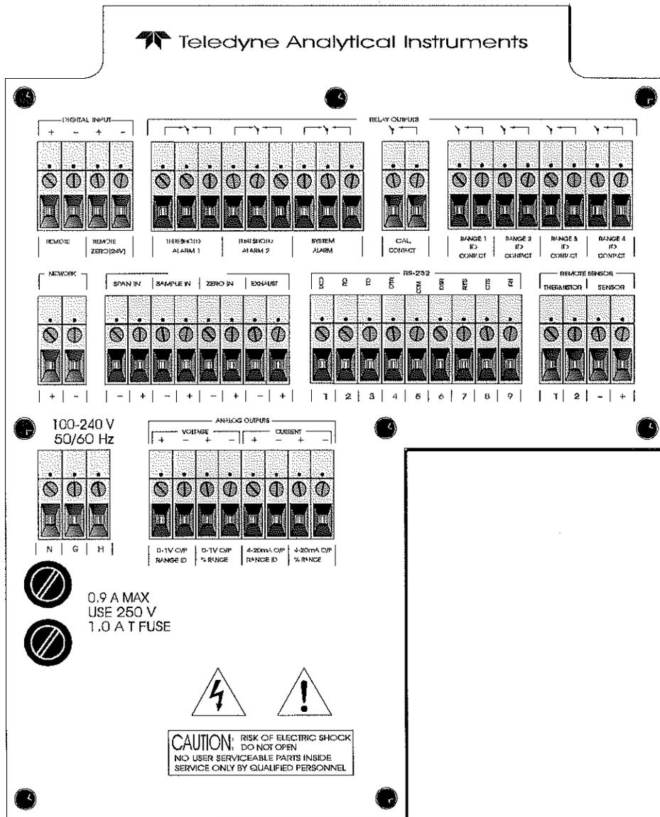
Figure 1-2: Model 3010PB Interface Panel
