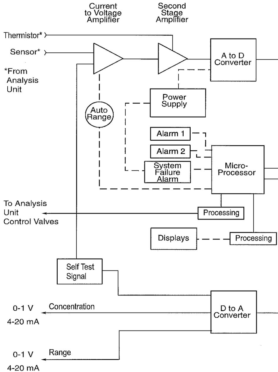
Figure 2-1: Block Diagram of the 3010PBC CU Electronics
