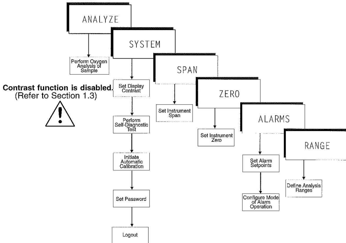
Figure 4-1: Hierarchy of Functions and Subfunctions
