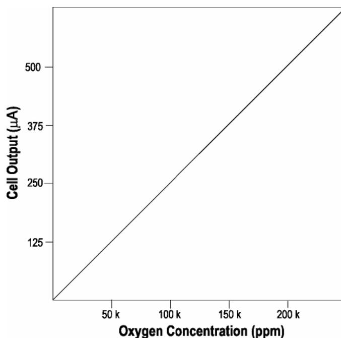
Figure 2-3. Characteristic MFC Input/Output Curve
