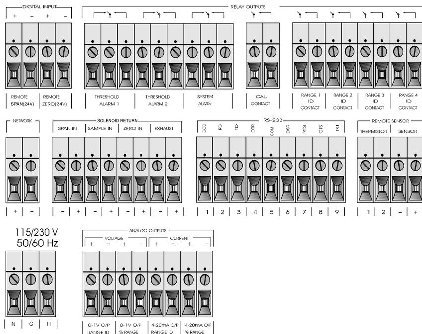
Figure 3-3: Electrical Connector Panel
