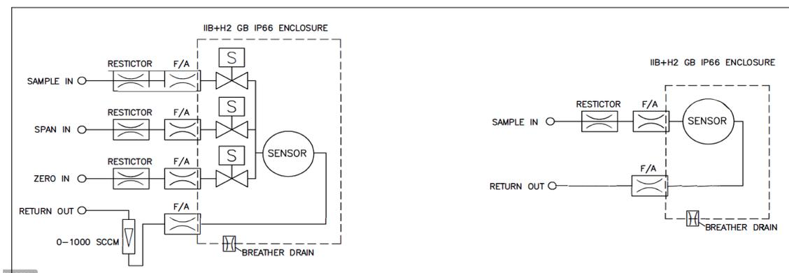
Figure 2-4: Flow Diagram
