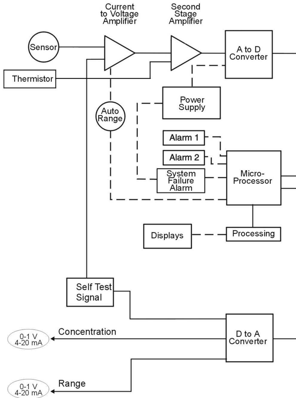
*Figure 2-5: Block Diagram of the Model 3020T Electronics*
