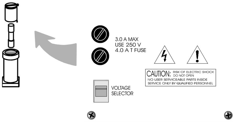
Figure 5-2: Removing Fuse Cap and Fuse from Holder
