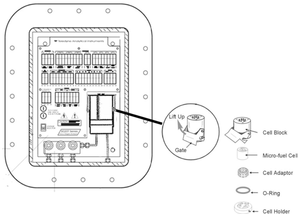
Figure 5-2: Sensor Replacement
