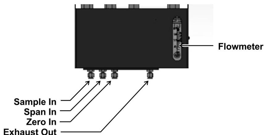
Figure 1-3: Model 3020T Optional Gas Connector Panel
