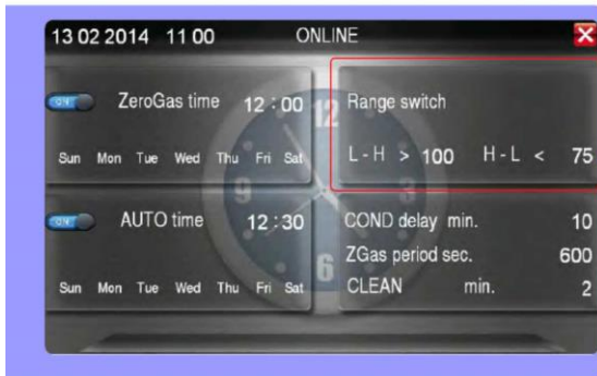
The threshold for automatic range switching can be set within the DUAL RANGE function
