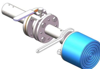
**Fig. 4.21 Disassembly diagram of transmitting/receiving unit**
