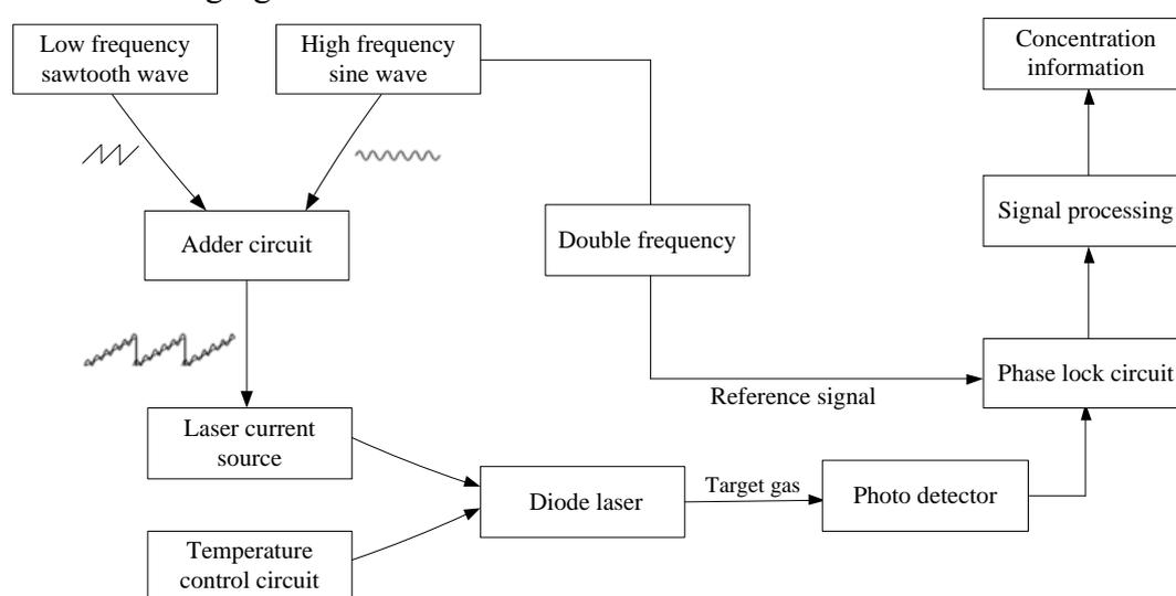
**Fig. 2.1 Functional block diagram of Diode Laser Gas Analyzer**
