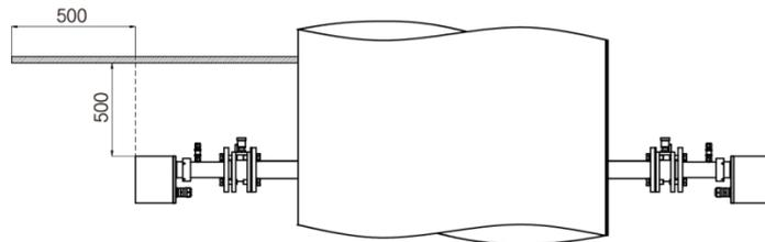
**Fig. 4.2 Installation diagram of sunshade**
