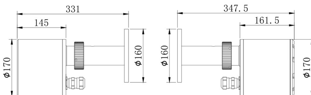
Fig. 3.1 Dimension diagram of LGA-4000Z Diode Laser Gas Analyzer
