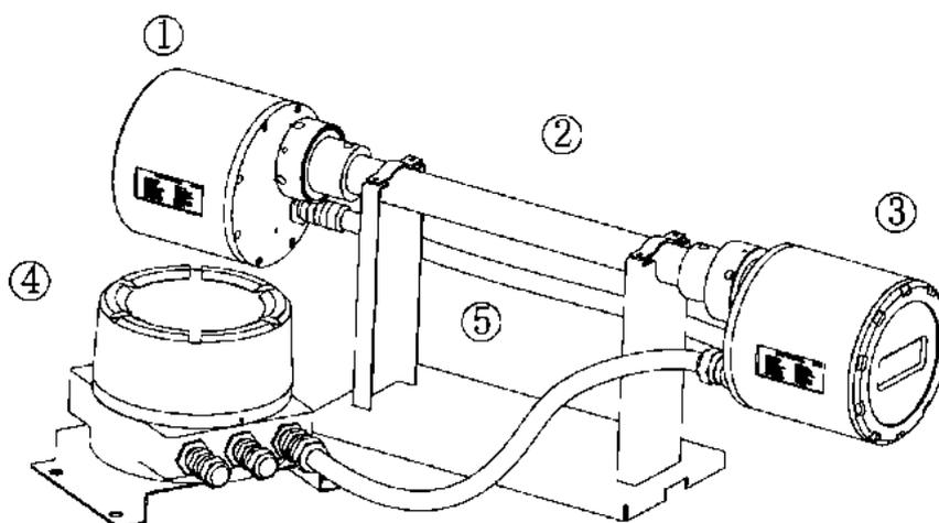
**Fig. 6.1 Install the transmitting and receiving unit on calibration gas chamber**
