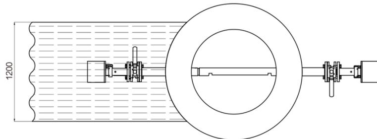
**Fig. 4.3 Top view of sunshade installation**
