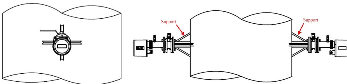
**Fig. 4.12 Standard support of instrument installation**
