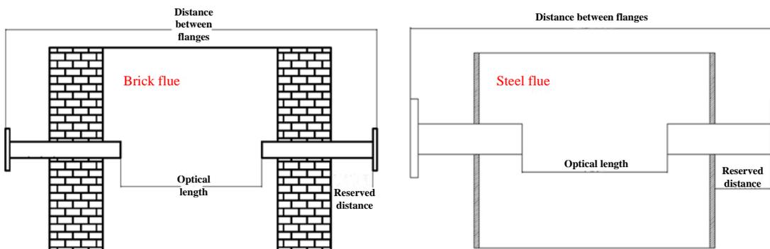
**Fig. 4.4 General flange installation**
