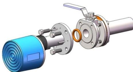
**Fig. 4.19 Instrument flange installation diagram**
