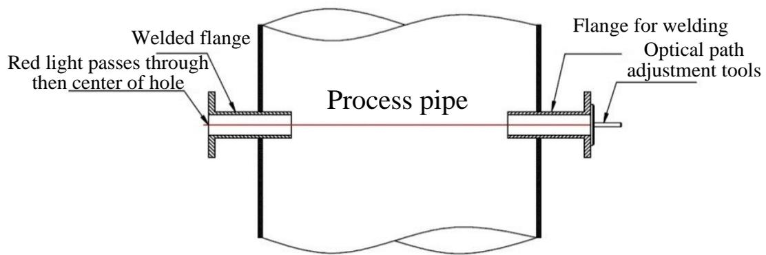
**Fig. 4.9 Flange installation 2**
