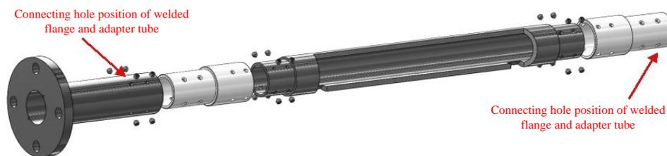
**Fig. 4.14 Connecting hole position of the welded flange and adapter tube**
