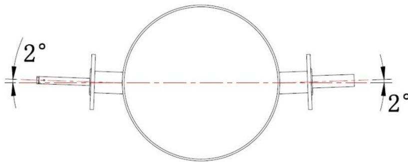
**Fig. 4.10 Permissible error of coaxiality**
