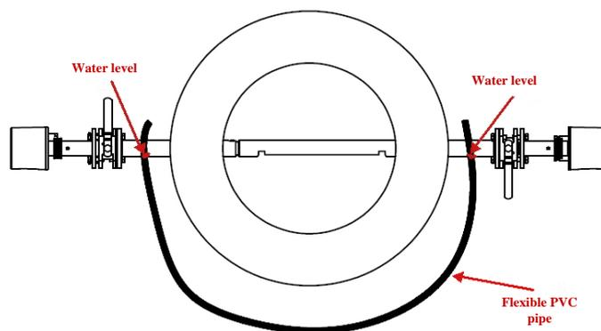
**Fig. 4.5 Use of leveling pipe**
