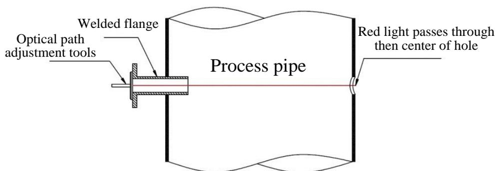
**Fig. 4.8 Flange installation 1**
