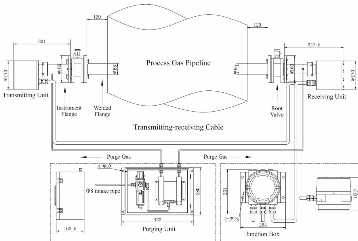
**Fig. 4.1 Installation diagram of LGA-4000Z Diode Laser Gas Analyzer**
