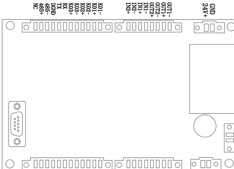
**Fig. 4.24 Wiring board diagram**
