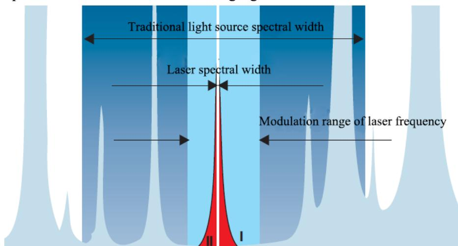
**Fig. 2.2 Schematic diagram of laser “single-line spectrum”**
