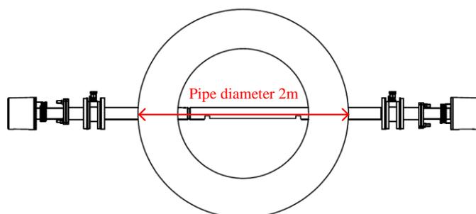
**Fig. 4.13 Pipe diameter**
