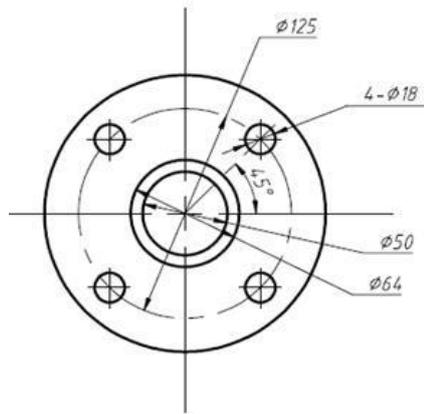
**Fig. 4.7 Welded flange dimension**
