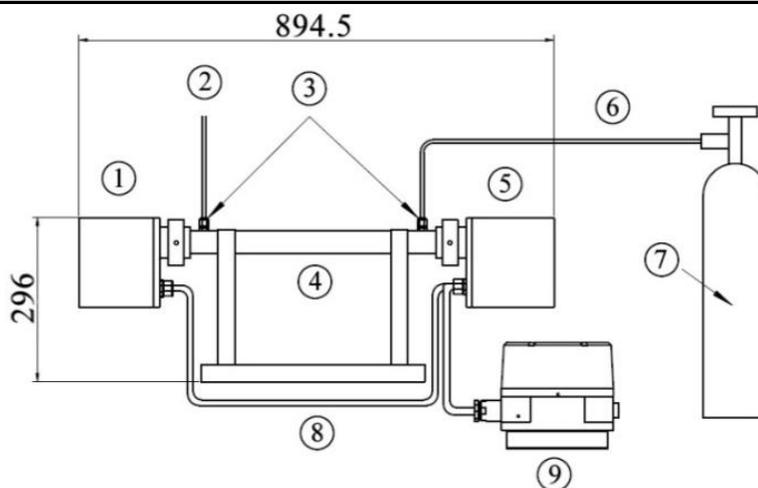
**Fig. 6.2 Calibration gas path connection**
