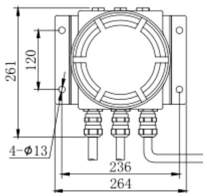
**Fig. 3.6 Dimension of junction box**
