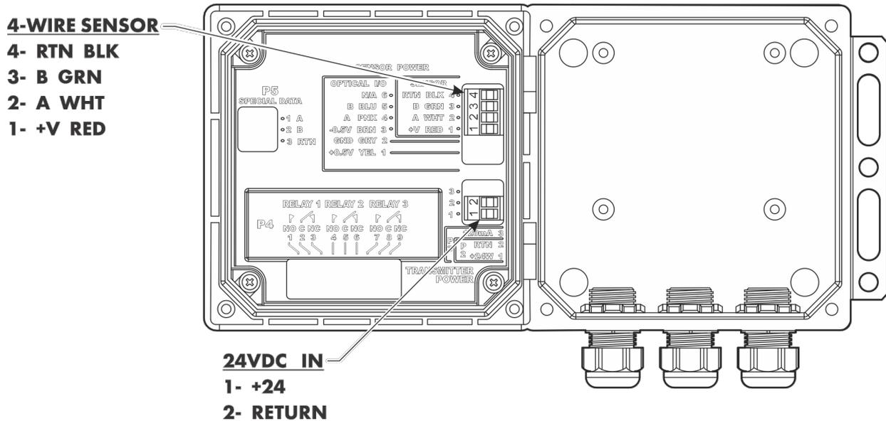
**Figure 3-5: Loop Powered Transmitter**
