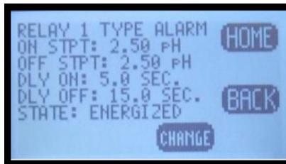
**Figure 4-28: Configure Alarm Relays**
