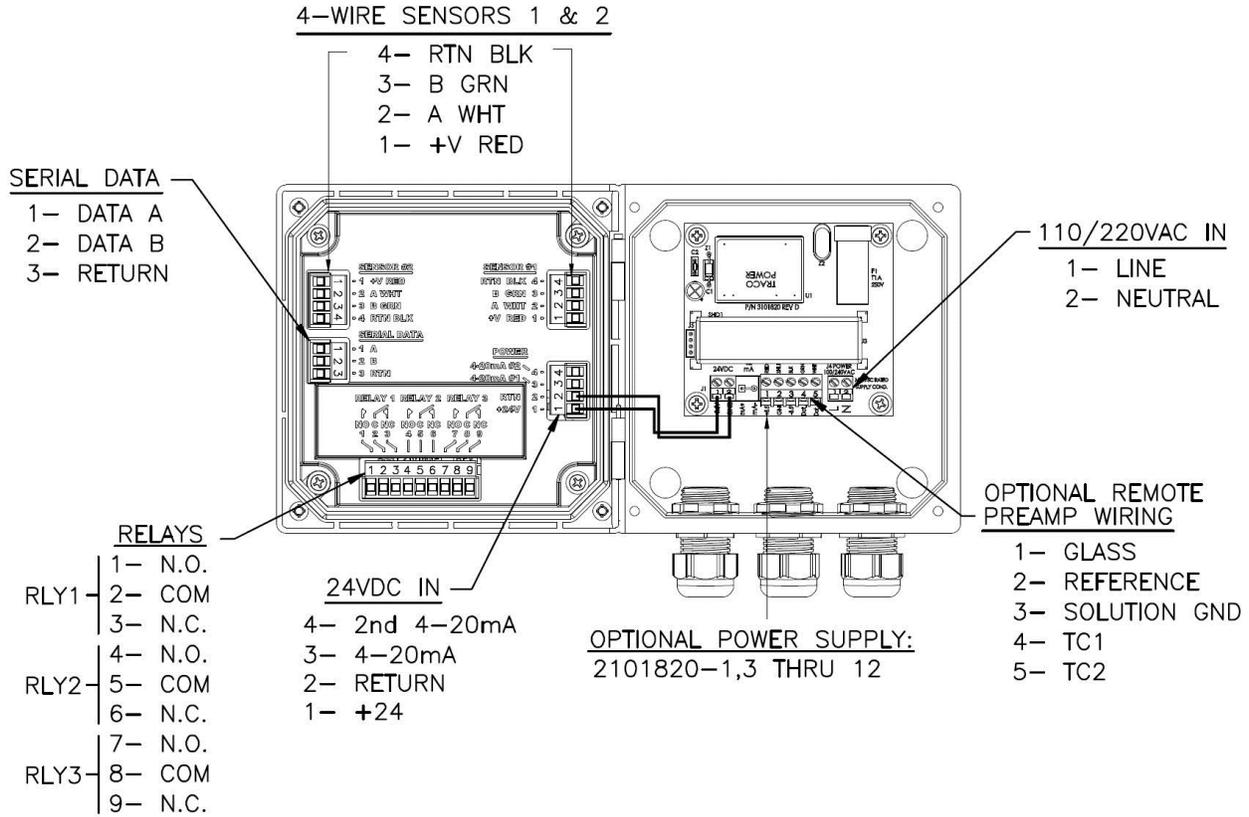
**Figure 3-6: 4-Wire Transmitter**
