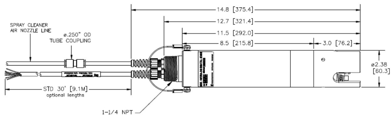
**Figure F-2: Ammonium NH<sub>4</sub>-N Dimensions**
