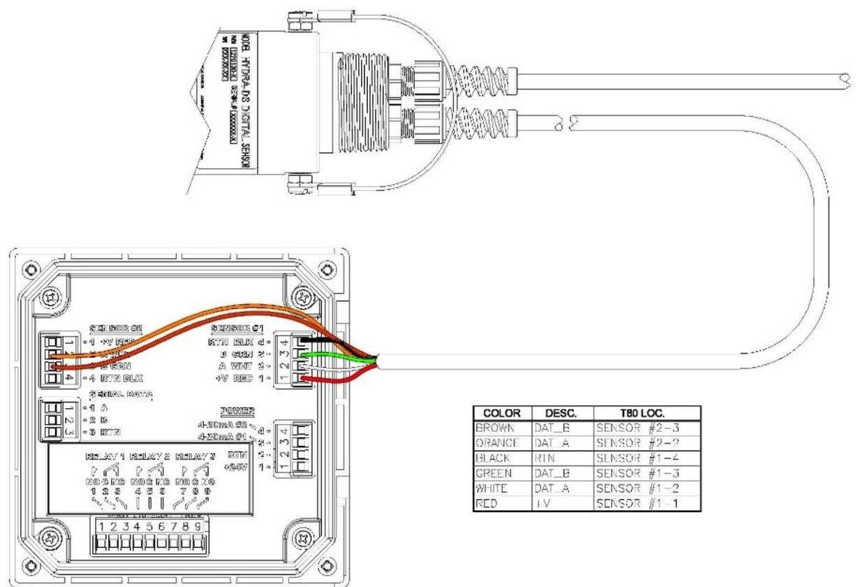
**Figure F-1: Wiring Diagram Ammonium NH<sub>4</sub>-N**
