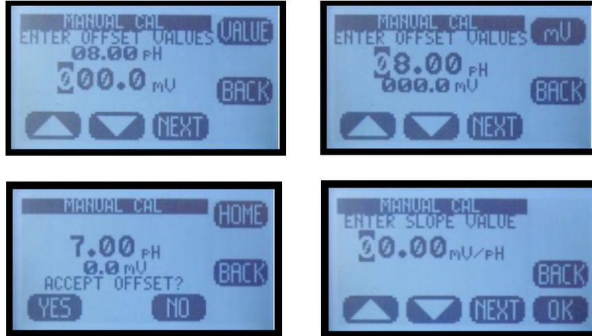
**Figure 5-1: MANUAL Calibration**
