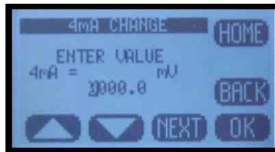
**Figure 4-26: Configure 4-20 mA Output Range, Screen 2**
