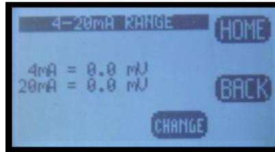
**Figure 4-25: Configure 4-20 mA Output Range, Screen 1**
