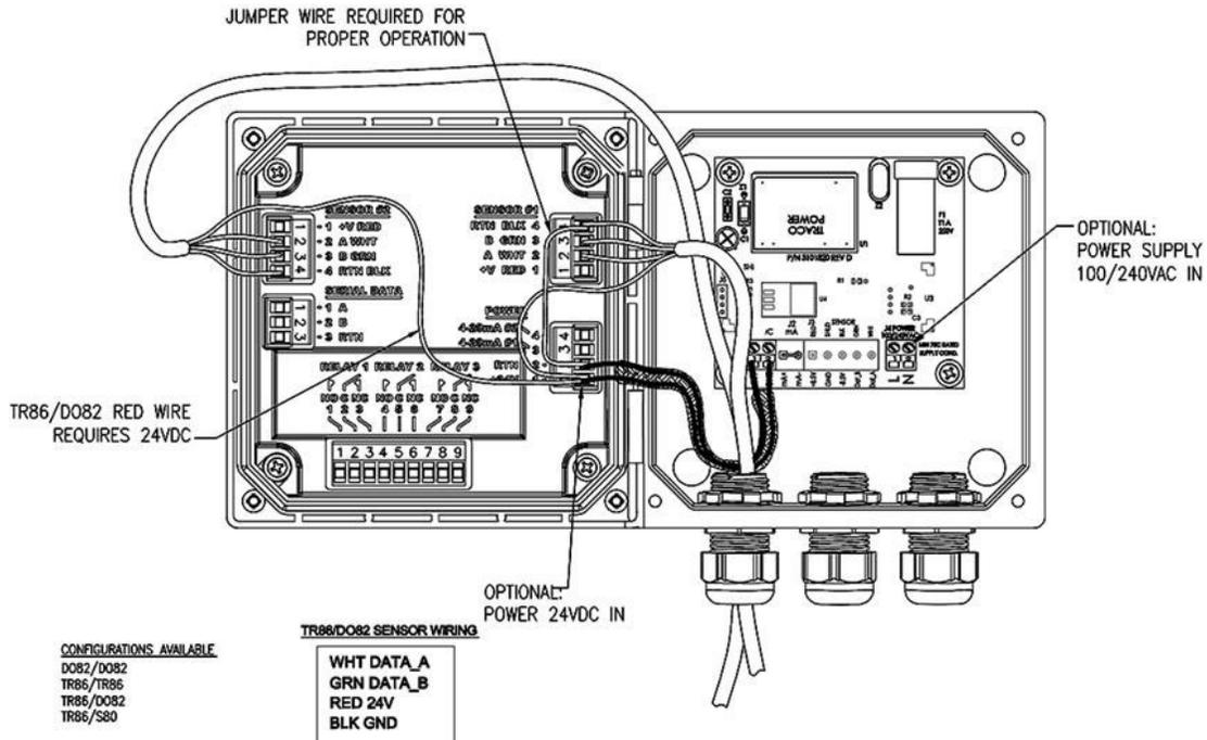
**Figure 3-7: 4-Wire Transmitter**
