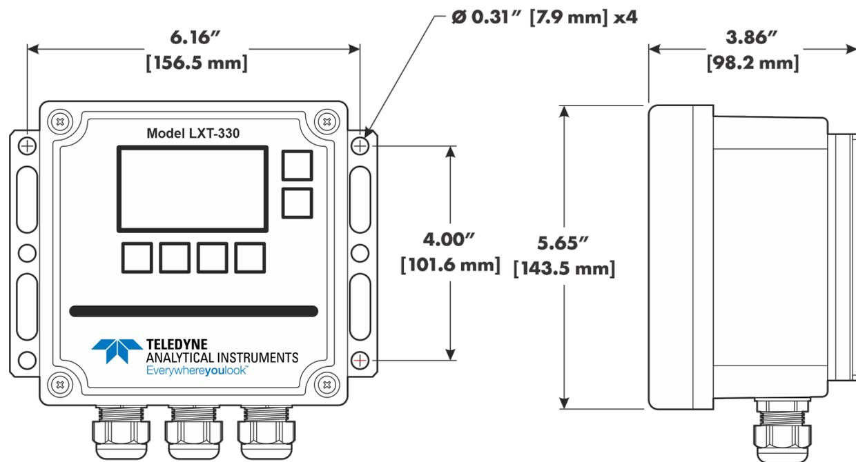
**Figure 3-2: Universal Mounting Bracket Dimensions**
