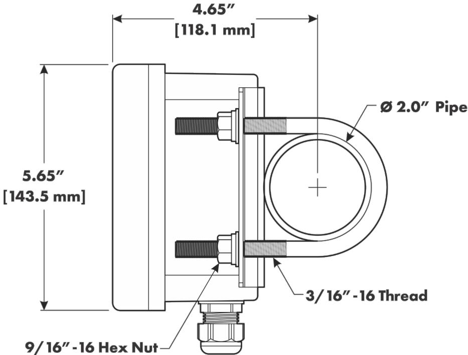
**Figure 3-3: Rail Mounting the Transmitter**
