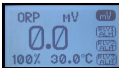
**Figure 4-33: mV Display Mode**
