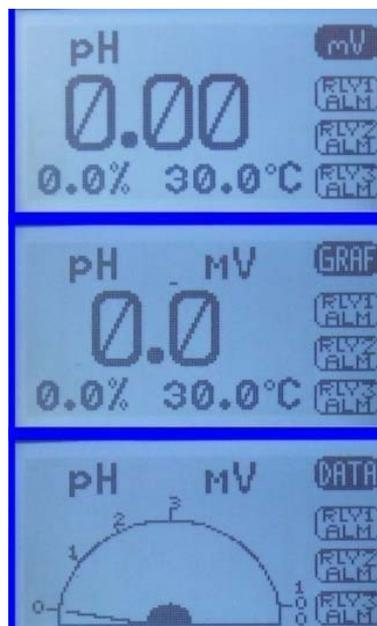
Each of the above screens also displays the condition of the optional Alarm Relays, black if energized and white if de-energized.
