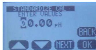
When the STAND key is pressed, the user is prompted to ENTER VALUE. The user enters the value they want the transmitter to read and press OK. The user is then prompted to accept the value, yes/no, and the calibration is complete. Standardizations are single point calibrations.
