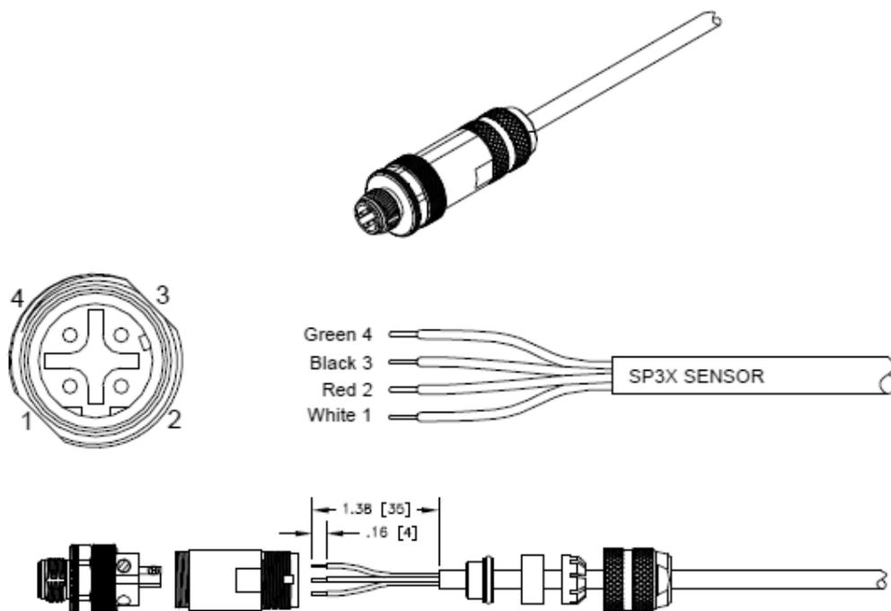
Figure 2-4: SP3X Sensor Connector Wiring
