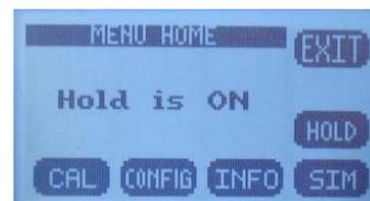
Actuating HOLD again turns the hold function off, Hold is OFF, displayed. The HOLD function remains ON until it is turned OFF. (See Time Out in CONFIG>XMTR>OUTPUT>HOLD).
