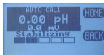
At the end of each calibration the Offset and Slope are displayed in the respective units, pH, mV, ppm, mg/l.
