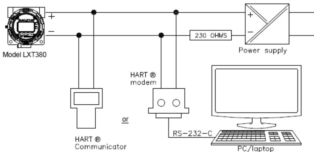
Figure 2-5: Wiring for HART® Communication
