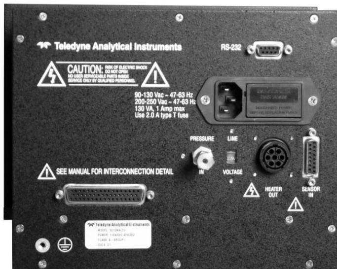
Figure 1-2 Rear Panel of Model 3010MA Control Unit
