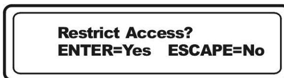
Pressing <Enter> will logout the current user and protect the system from unauthorized changes to parameters. All users will still have access to the SELF-TEST function and the instrument will function normally in *Analyze Mode*. If you press <Escape>, the current password will still be in effect and the user has not logged off.
