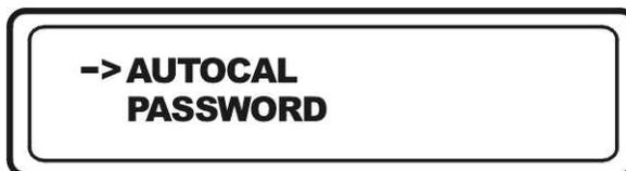
**<▲ ▼>** If the arrow is not adjacent to the AUTOCAL menu item, use the ▲ ▼ keys to move the arrow to the proper position.
