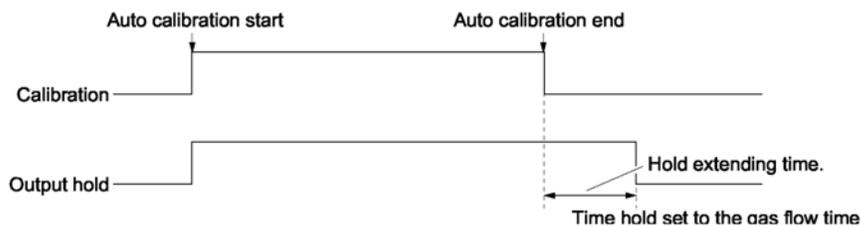
*Figure 3-11: Output Hold for Auto Calibration*
