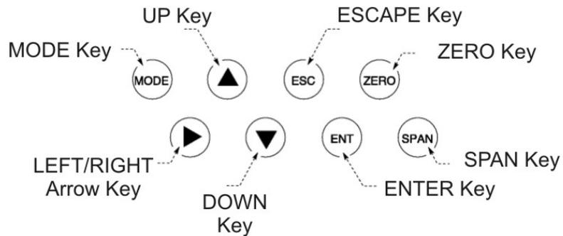
Figure 3-2: Interface Keys on the Front Panel
