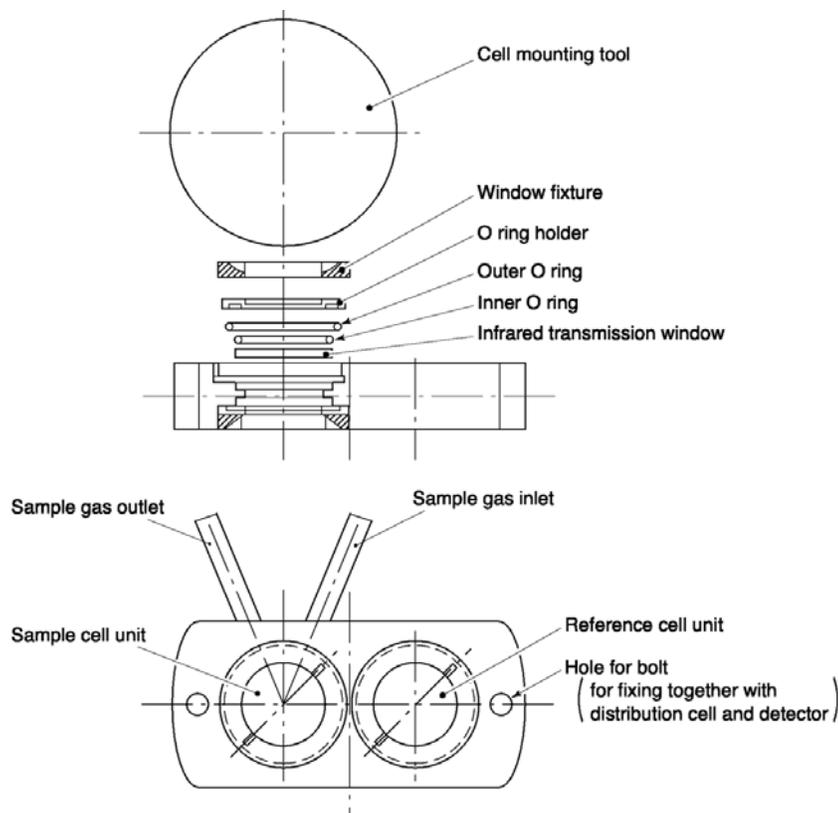
Figure 4-6: Cell Block Assembly
