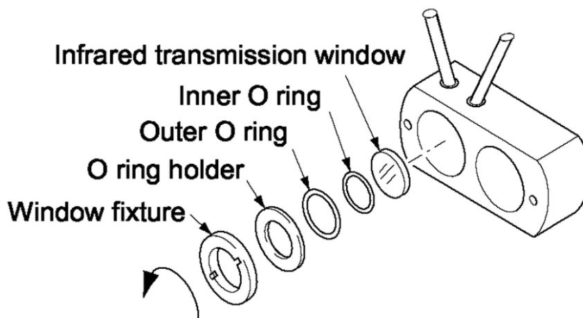
Figure 4-4: IR Window Assembly
