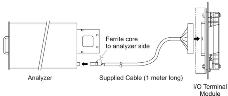
Figure 2-11: I/O Cable Connection
