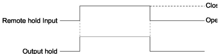
*Figure 3-12: Output Hold for External Hold*
