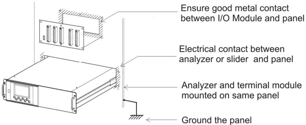
Figure 2-3: Mounting the I/O Module
