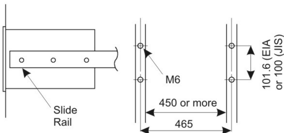
Figure 2-1: Slide Rail Mounting Dimensions
