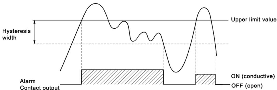
Figure 3-6: Hysteresis Example for a High Limit Alarm
