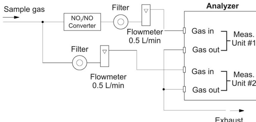
Figure 2-6: External Piping with Two Pair of Inlet/Outlet (1)
