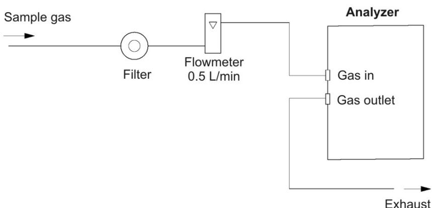
Figure 2-5: External Piping with Single Inlet and Outlet
