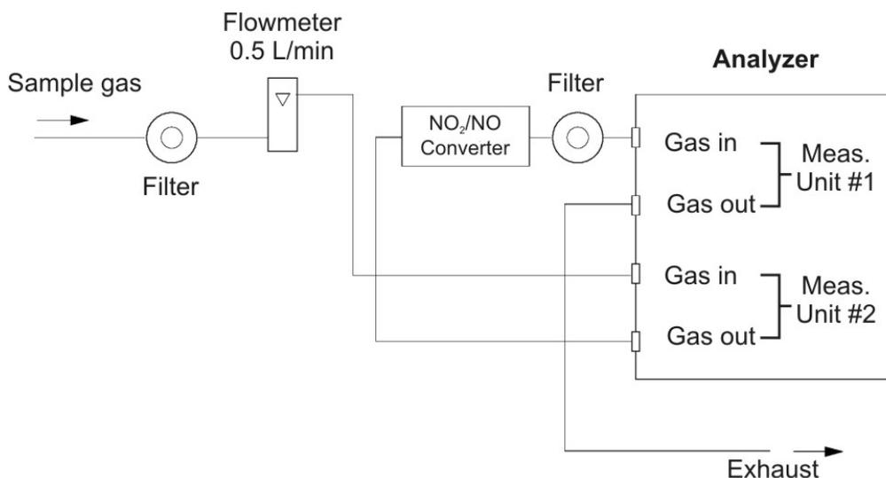
Figure 2-7: External Piping with Two Pair of Inlet/Outlet (2)
