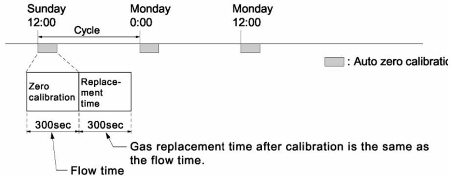
Figure 3-8: Example Auto Zero Calibration
