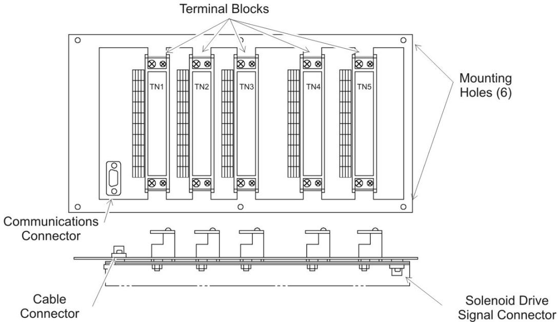
Figure 2-2: Input/Output Terminal Module
