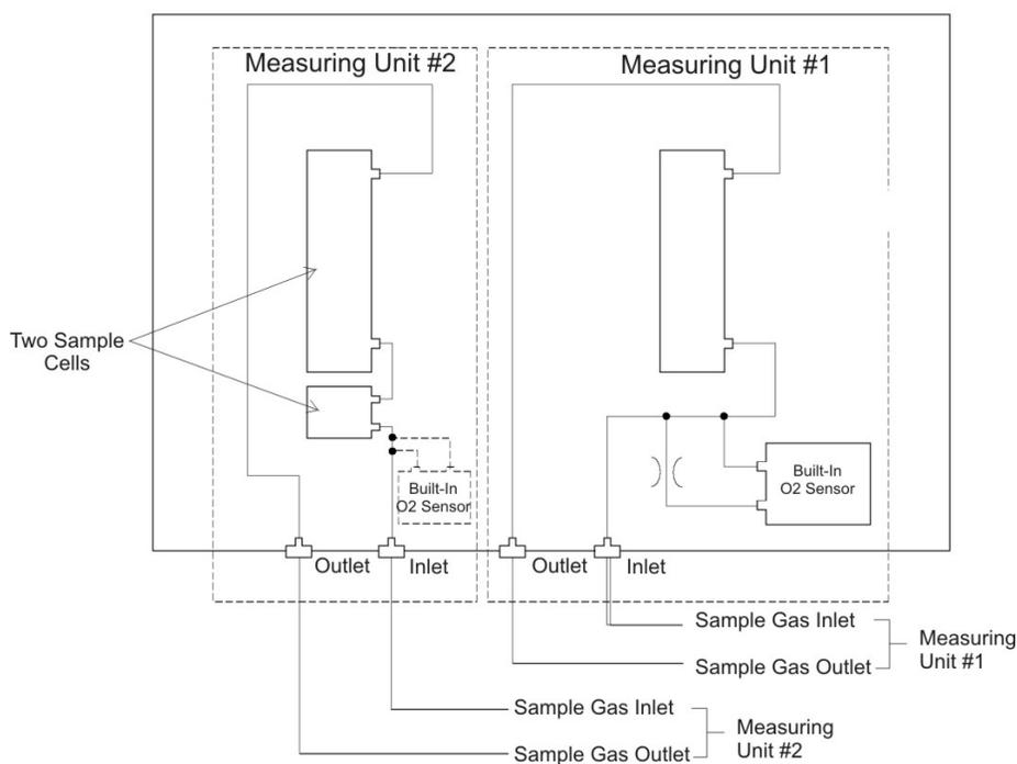
Figure 2-4: Internal Piping with Single or Dual Measuring Units
