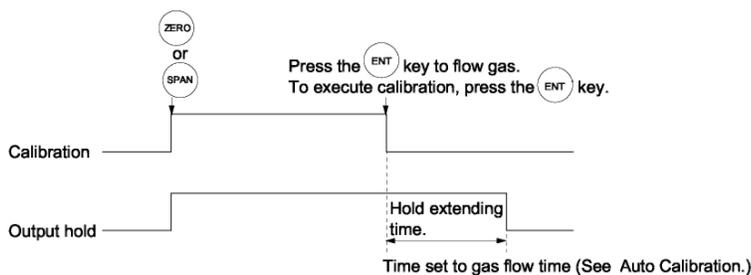
Figure 3-10: Output Hold for Manual Calibration
