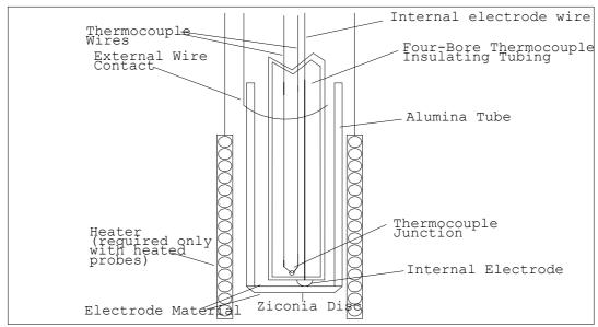
Fig 2.1 Schematic View of a Sensor Assembly
