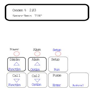
Figure 4.1 Operator's Panel
