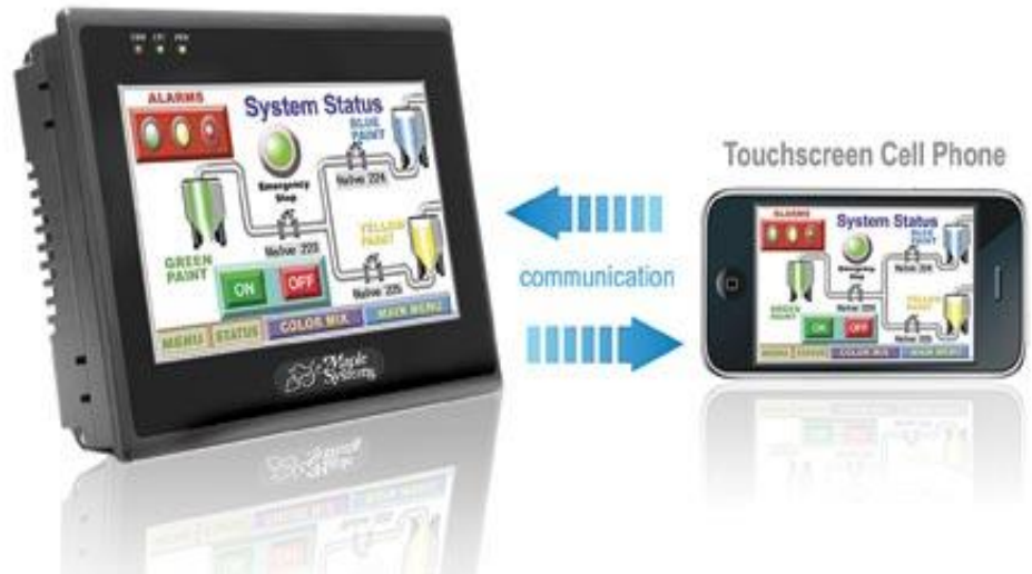
Figure 1-1: Communication between HMI and Phone
