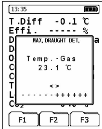
Draught detection is only available for the measurement of the flue gas temperature in the Flue Gas menu.
