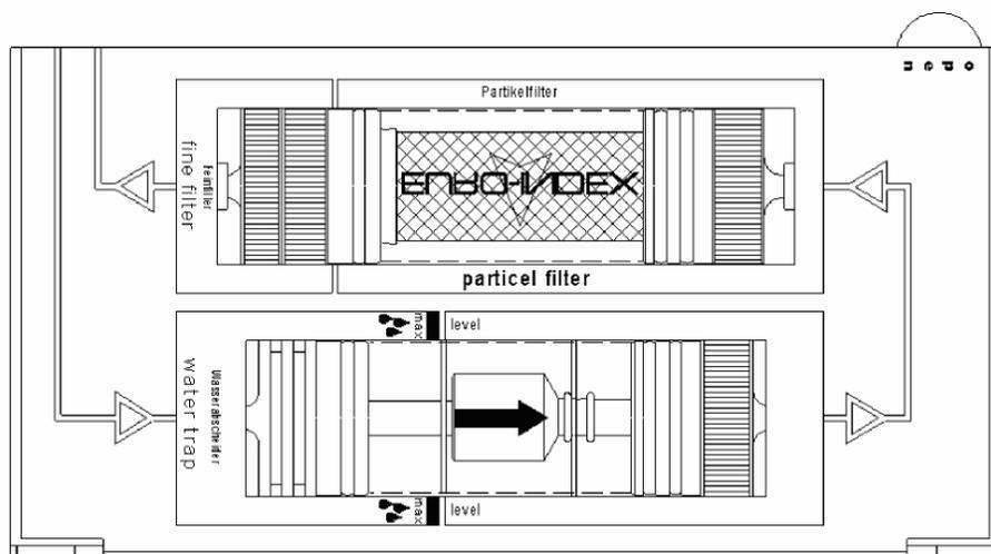
Figure 2-4: Gas Conditioning System
