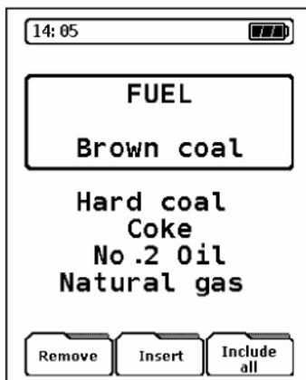
From this screen you can remove a fuel from the list, add a fuel to the list or include all the fuels programmed into the analyzer memory including those that have been removed.
