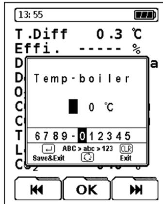
*Note: When the input menu for the extended data (Smoke-no., oil derivatives and boiler temperature) is closed all data that has been confirmed with the ENTER button will be stored in the measurement protocol. Inputs of data that have been cancelled will be discarded.*
