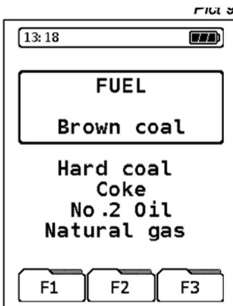
At this point, either the fuel in the framed box can be chosen or any another fuel from the database of fuels in memory. The selected fuel has to be in the framed box.
