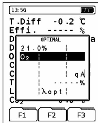
*Note: If both bars extend to the optimal fuel-air relation (the gap indicated  $\lambda_{opt}$ ) the firing facility in question is set correctly.*
