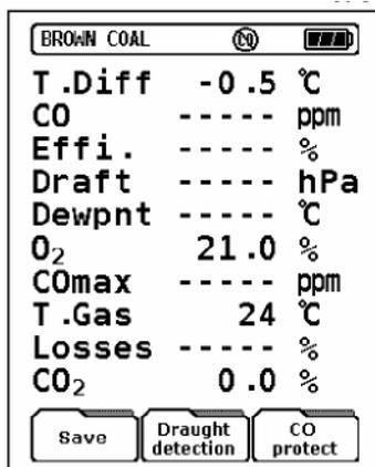
If the CO-flushing-pump starts automatically due to an excess concentration of CO it cannot be switched off manually until the CO-concentration falls below a factory preset value.
