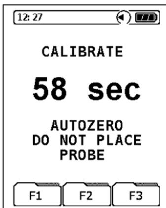
The instrument begins an automatic calibration cycle which takes approximately 60 seconds from a cold start. If a restart is performed from the Measurement screen, the calibration process only takes 10 seconds. The instrument probe should not be attached during this calibration.
