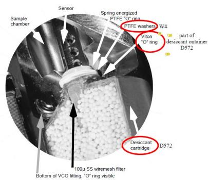
Bottom view of 8800P with cover open. The sample chamber and desiccant cartridge are shown cut open to facilitate an understanding of the mechanism and how it is assembled.
