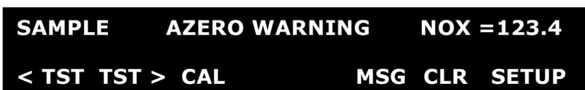
The analyzer will also issue a message to the serial port and cause the red FAULT LED on the front panel to blink.
